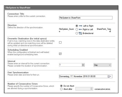
Figure 16 - Example: File System to SharePoint set to run once a day at 01:00 AM
