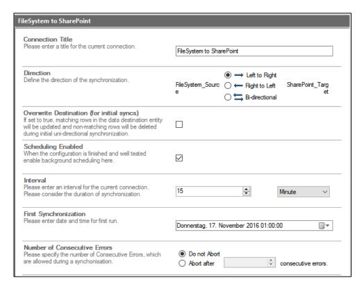
Figure 17 – Example: File System to SharePoint set to run every 15 minutes
