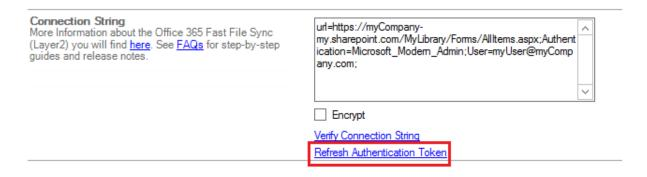
Figure 80 - Link in the UI to refresh the authentication token for Microsoft\_Modern\_Admin authentication
